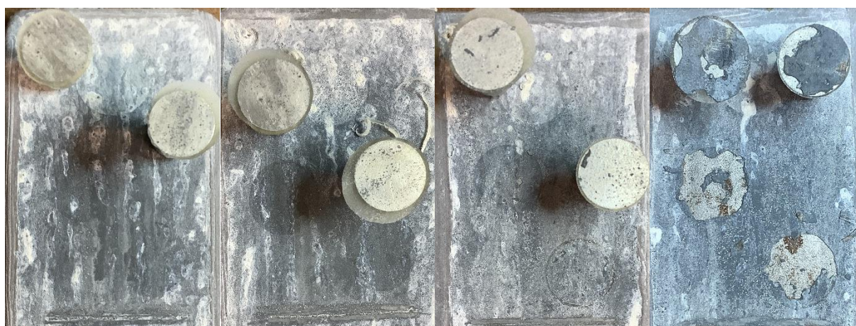
Figure 6. Pull off on panels 1 - 4 (left to right) after qualification testing.
