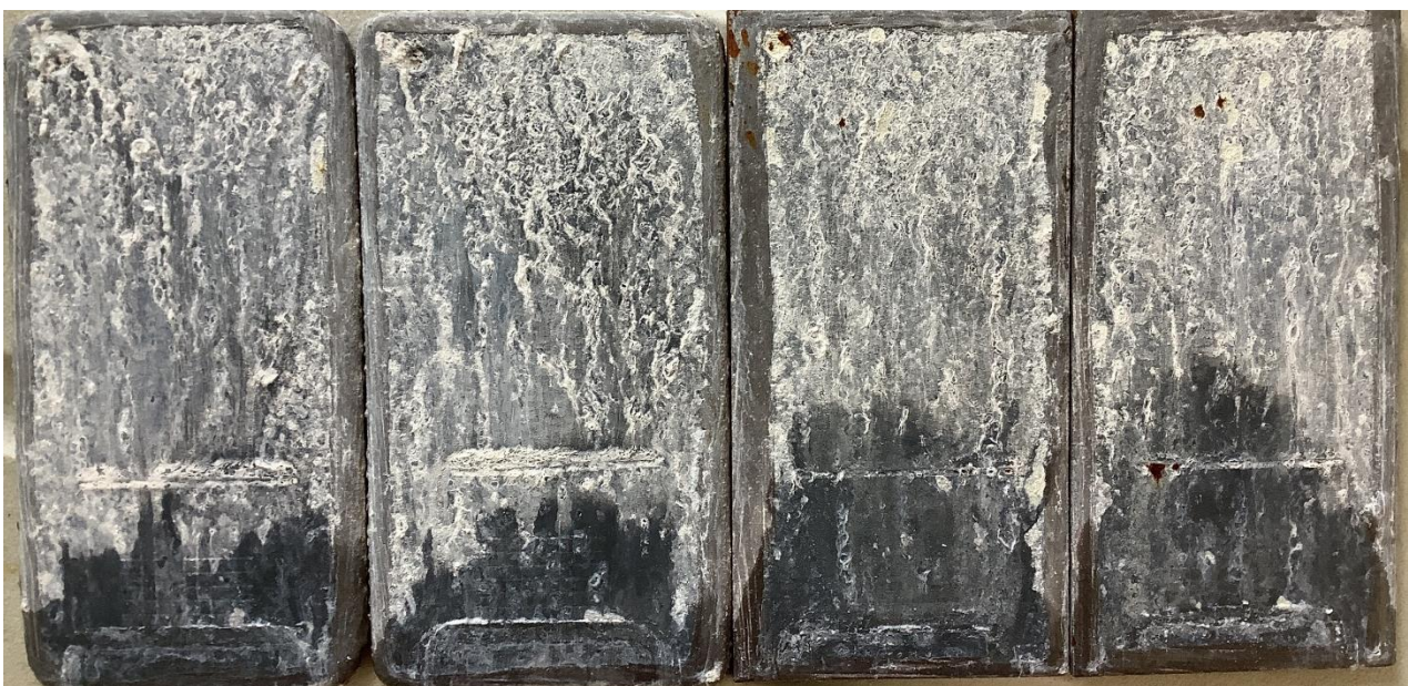
Figure 5. Panels 1 - 4 (left to right) at 1440 hour of salt spray testing.
