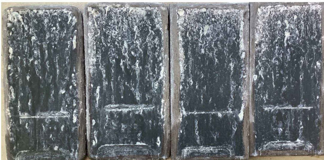
Figure 3. Panels 1 - 4 (left to right) at 645 of salt spray testing.
