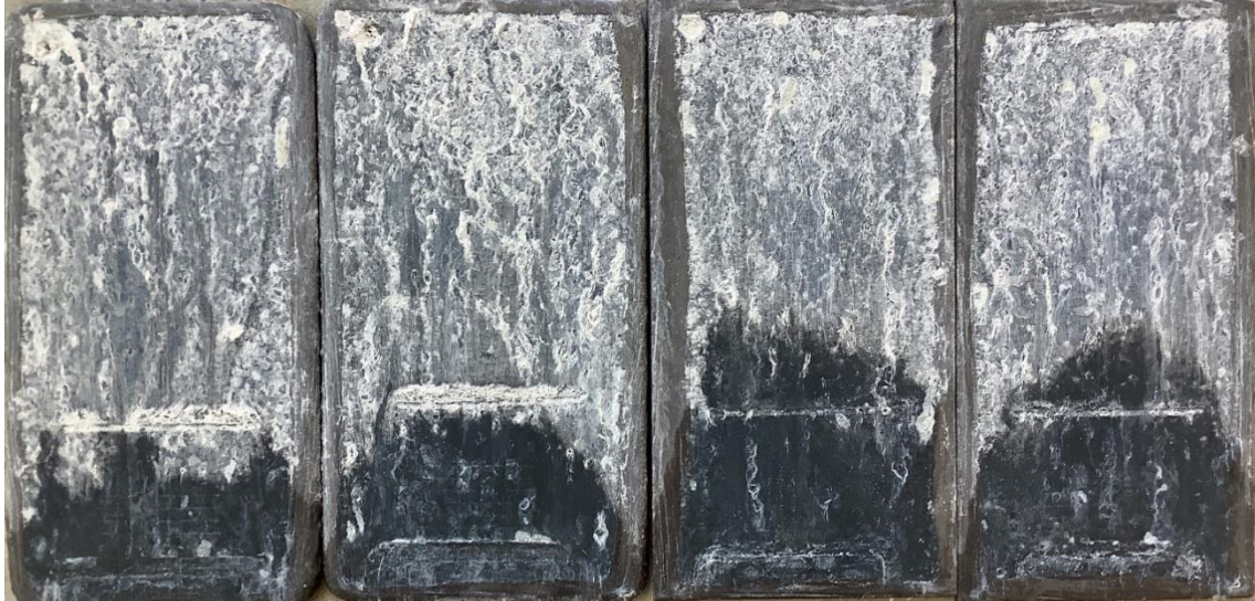
Figure 4. Panels 1 - 4 (left to right) at 1000 hour of salt spray testing.
