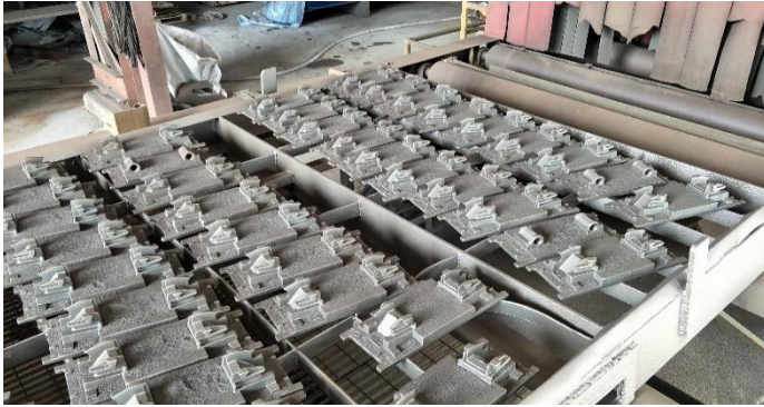
Baseplates after passing the Autoblaster Machine using angular metallic abrasives.
