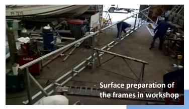
System: Sandblasting to degree SA 2.5 ZINGA 2 x 60 µm DFT
