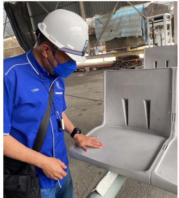
Quality control of the surface preparation before application of the 1st ZINGA layer.
